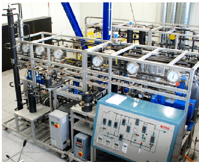
Fig. 8. The laboratory plant of solid-supercritical carbon dioxide extraction
